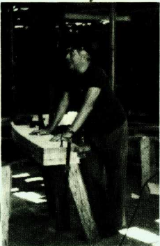
ABOVE: Captain Francis “Flyer” Santos laminating the stem of the “Rose Dorothea” in his workshop at Flyer’s Boatyard.
