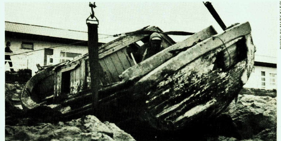
After the third attempt, the boat was cracked out of the mud and it was discovered the keel was intact.
