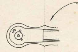
DETAIL of REAR OF HAND SHOWING, COLLAR W/SET SCREWS (2), PLATE W/"88" NUMERAL EMBOSSED, AND RT. ANGLE RIBS
